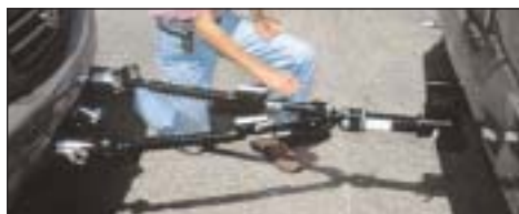
ONCE THE PINS ARE IN, THE MOTORHOME IS DRIVEN AHEAD SLOWLY (OR DINGHY BACKED) TO LOCK THE ARMS IN POSITION.
