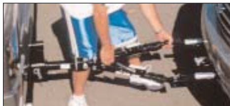
TO HOOK UP USING A TELESCOPING TOW BAR, DINGHY VEHICLE ONLY NEEDS TO BE NEAR CENTER AND MID-LENGTH OF BAR.
