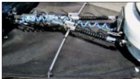
AN RV UNDERSKIRT WILL KEEP TOWING APPARATUS CLEAN — AND IT ALSO HELPS PROTECT THE FRONT OF THE TOWED VEHICLE FROM ROAD DEBRIS.
