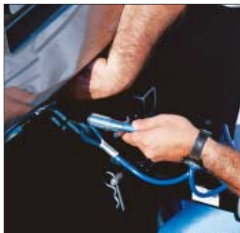
PLUG RECEPTACLES ADDED TO DINGHY AND MOTORHOME ALLOW EASY HOOKUP OF ELECTRICAL CONNECTOR FOR TAILLIGHTS, TURN SIGNALS AND SUPPLEMENTAL BRAKING SYSTEM.
